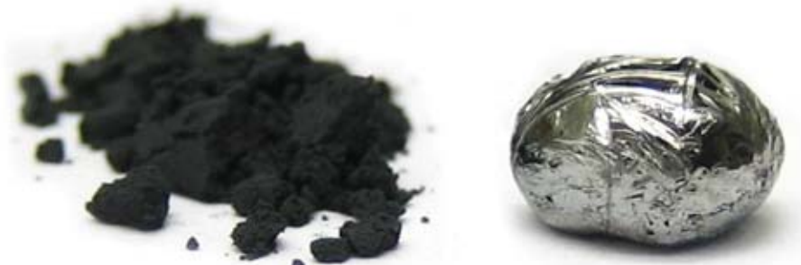
MAKING ULTRAHARD MATERIALS usually requires extreme pressures. Heat alone can convert rhenium diboride powder (left) into a pellet (right) hard enough to scratch diamond.
